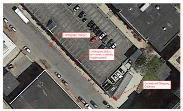
Figure 11 Elm St Pulse On-Route Charger Layout Option
