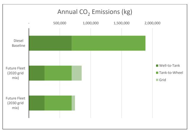
Figure 15 Graph of CO<sub>2</sub> Emissions Estimate Results
