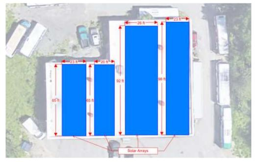
Figure 12 13 Pomerleau Facility Proposed Solar Array
